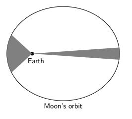
The shaded areas are equal and so are traced in equal times.
